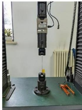
Fig.9: Tension/length of cable test
